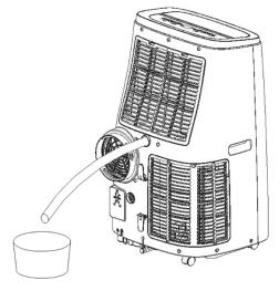
${\bf 2.Next, insert\ the\ drainage\ tube\ into\ the\ connection\ tube.}$
