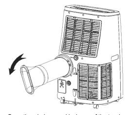
Connect the round window fitting (1) to the end of the hose then the end fitting for the window (2)
