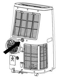
Remove the cap by turning it anti-clockwise then remove the plug.
