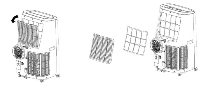
Use a vacuum cleaner to remove any dust from the upper filter removed. Should this not be sufficient, wash the filter with lukewarm water and neutral detergent (if necessary), rinse it with cold water then leave it to dry naturally before putting it back in place. After putting the filter back in place, close the grille and resume use of the air conditioner.
