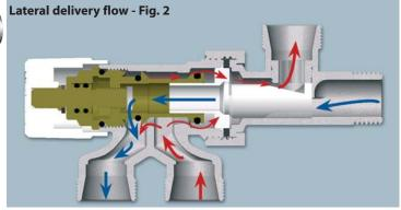
The connection with external probe permits fluid inlet into the upper part of radiator and fluid outlet into the lower section, thus guaranteeing optimal heat distribution.
