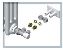
Example of installation of adapters for multilayer pipe
