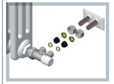
Example of installation with sealing kit for copper pipe. (The illustration shows the connection up to  $\emptyset$  14 complete with a brass pipe guide washer - not needed for  $\emptyset$  15 and  $\emptyset$  16 mm)
