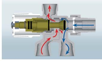
**24x19 connections** for copper, plastic and multilayer pipe; 35 mm centre line between ports
