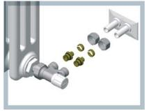
Example of installation of adapters for plastic pipe
